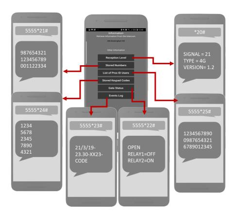
This screen allows the engineer or manager to be able to check multiple things on the intercom. Please note the following points..
